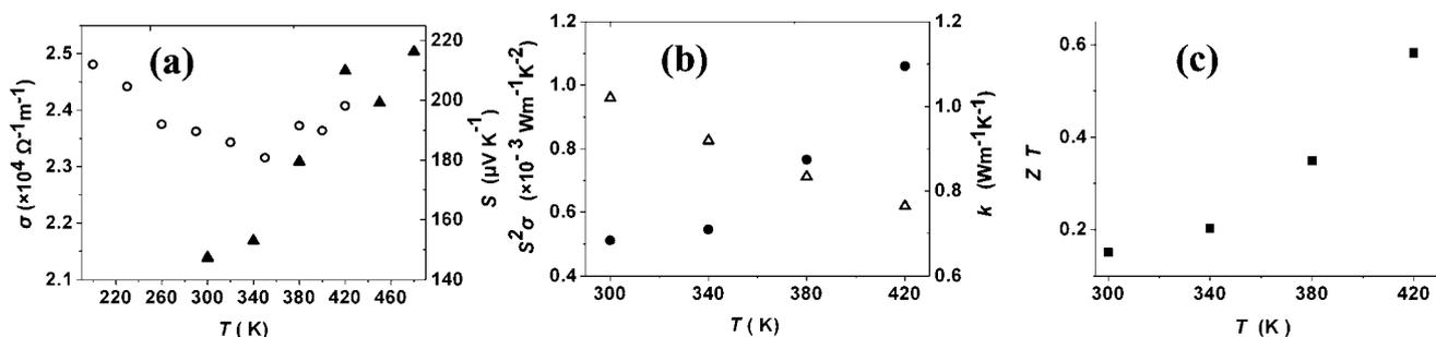
**Fig. 3** The temperature ( $T$ ) dependences of thermoelectric properties of the  $\text{Sb}_2\text{Te}_3$  nanosheet bulk sample sintered by SPS: (a) electrical conductivity  $\sigma$  (○) and Seebeck coefficient  $S$  (▲); (b) power factor  $S^2\sigma$  (●) and thermal conductivity  $\kappa$  (△); (c) the dimensionless figure-of-merit  $ZT$  (■).
