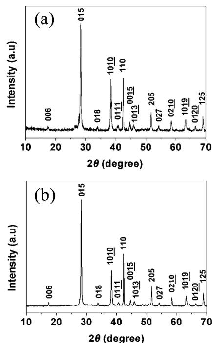
**Fig. 1** XRD patterns. (a) The  $\text{Sb}_2\text{Te}_3$  powder prepared by the microwave solvothermal method using  $\text{SbCl}_3$ ,  $\text{Na}_2\text{TeO}_3$  and hydrazine hydrate in ethylene glycol at 200 °C for 15 min; (b) the  $\text{Sb}_2\text{Te}_3$  nanosheet bulk sample sintered by SPS in vacuum at 270 °C for 6 min.
