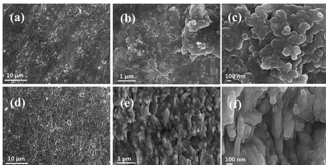
**Fig. 4** SEM micrographs of  $\text{Sb}_2\text{Te}_3$  nanosheet bulk samples after measurements of all thermoelectric properties. (a–c) Surface plane of the samples, and (d–f) cross-section of the samples.
