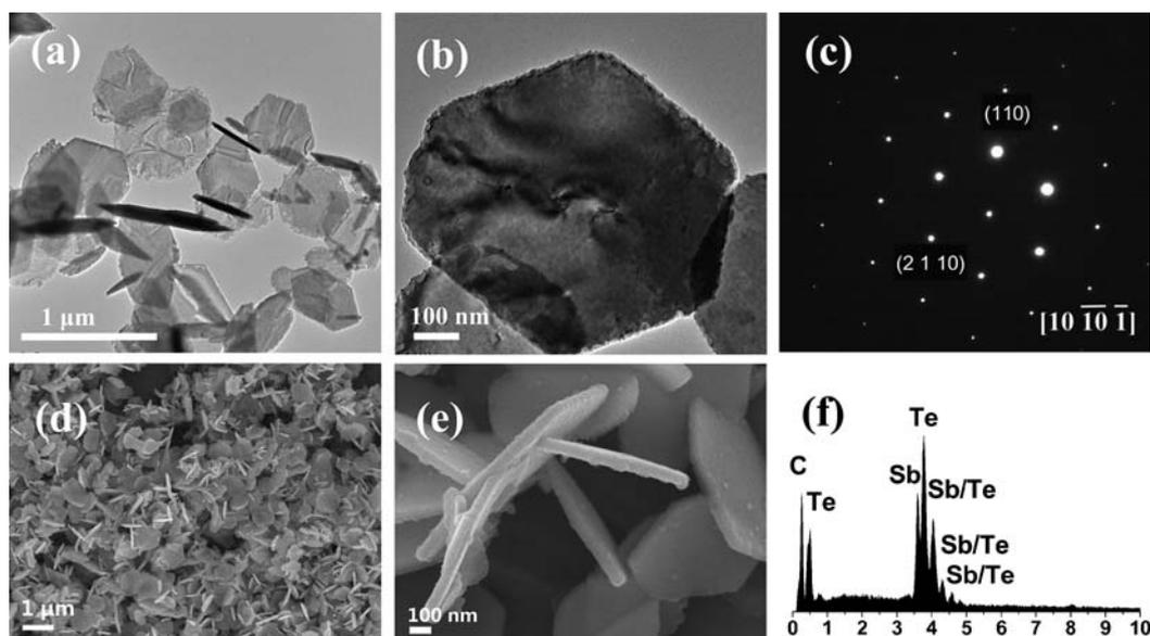
**Fig. 2** TEM and SEM micrographs and EDS of  $\text{Sb}_2\text{Te}_3$  nanosheets prepared by the microwave solvothermal method using  $\text{SbCl}_3$ ,  $\text{Na}_2\text{TeO}_3$  and hydrazine hydrate in ethylene glycol at  $200^\circ\text{C}$  for 15 min. (a,b) TEM micrographs; (c) SAED pattern taken from a single nanosheet; (d) low-magnification SEM micrograph; (e) high-magnification SEM micrograph; (f) EDS.
