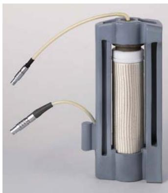
The piezoelectric crystal, like electronic balance, is installed at the bottom or at the top of the vessel and delivers pressure parameter via electrical signal.
