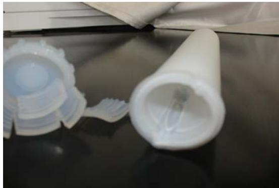
Automatic release valves are deformed and broken after several escaping and cannot be restored.
